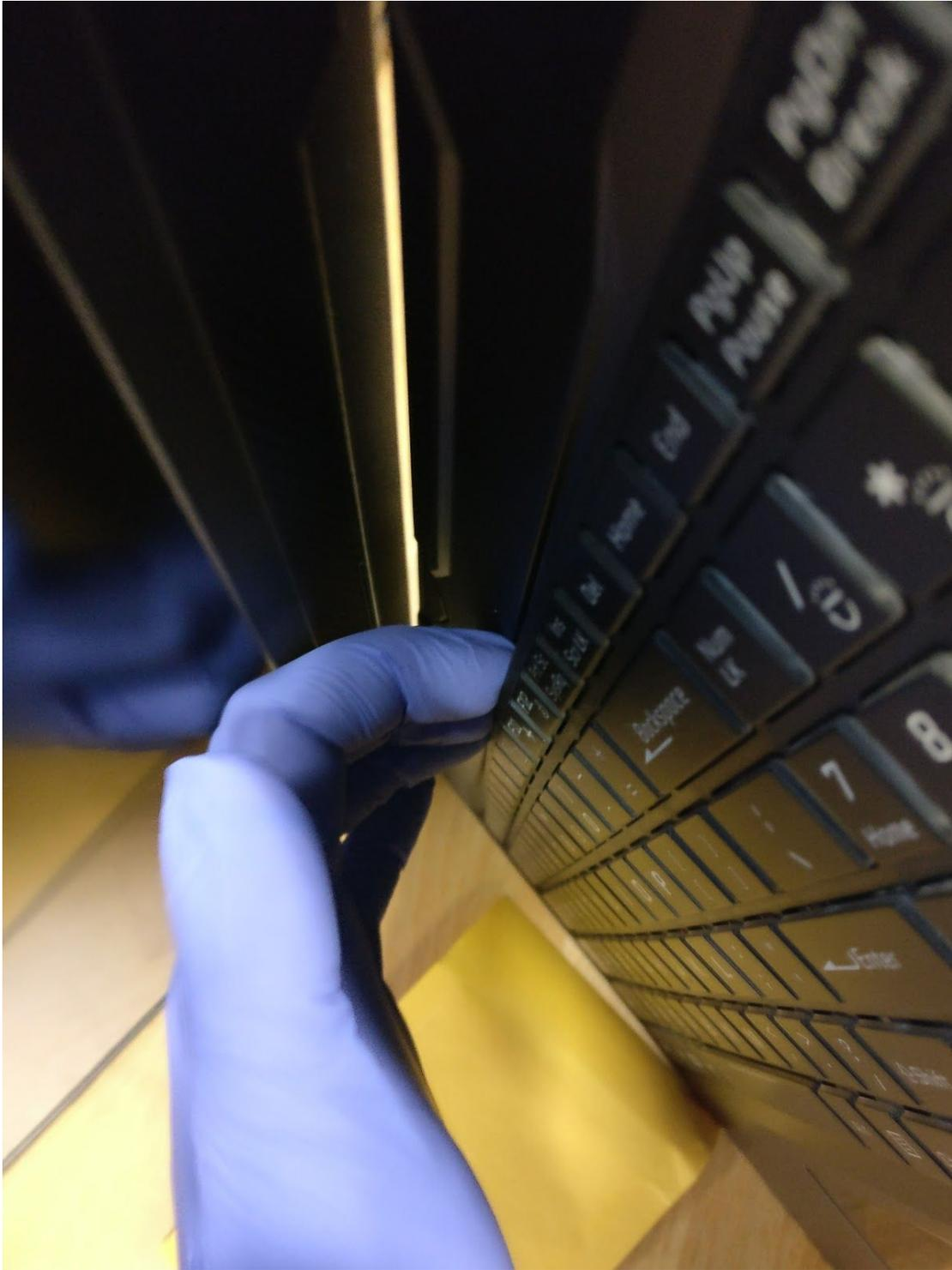
4. Flip the keyboard over and rest it on the trackpad. Pull the large ribbon cable out of the connector. The smaller ribbon cables have latches. Gently pull it forward to release the connector, then remove the ribbon cables.
