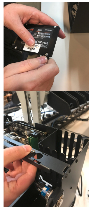
Fig. 31: (above and below-right) Sequence of shots showing the removal and/or replacement of 2.5" drives in the Thelio drive cage.
