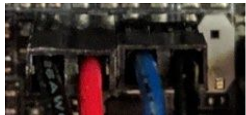
Fig. 16: Motherboard power button and Thelio Power Button connections.
