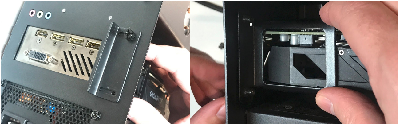
Fig. 28: Replacing the thumbscrews and GPU Bracket.
