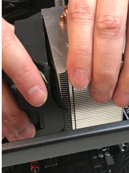
Fig. 33: Removing the CPU Cooler Fan from the Heat Sink.
