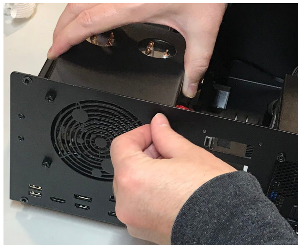
Fig. 20: Replacing the CPU Cooler Shroud and thumbscrews.
