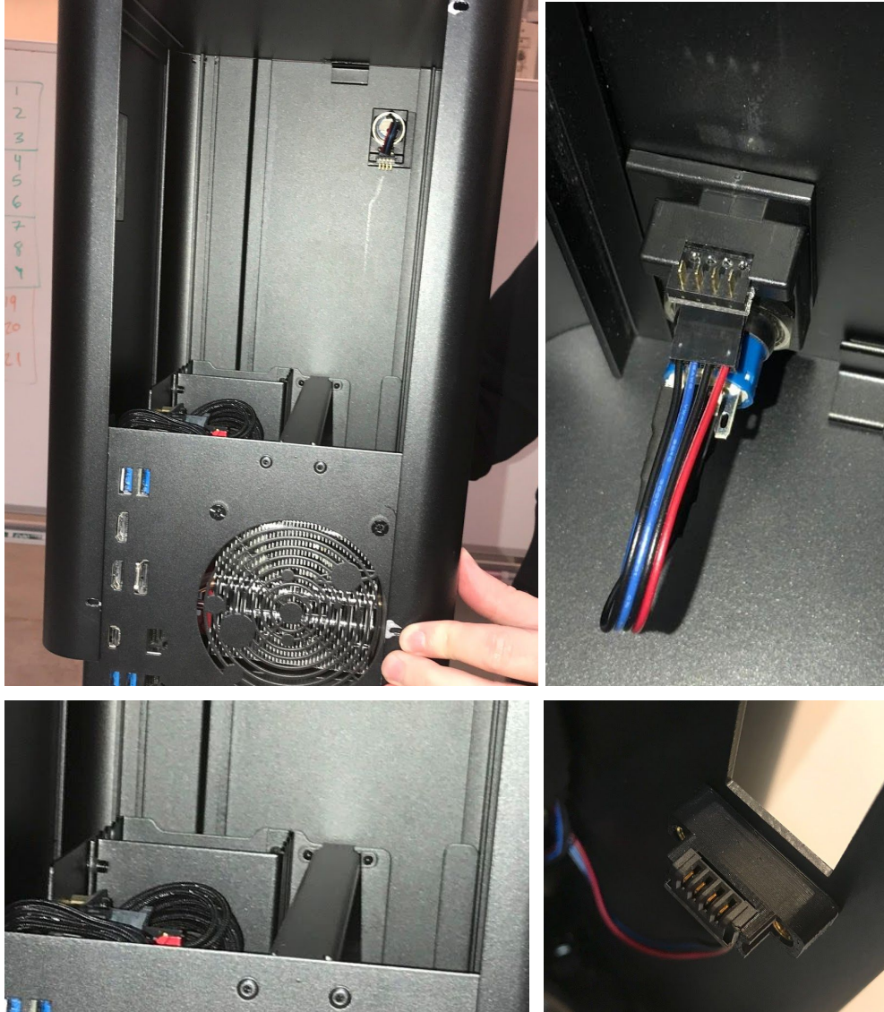
Fig. 11: Aligning the Thelio Top Case for replacing (left, top and bottom). Detailed view of Thelio internal switch (right, top and bottom).
