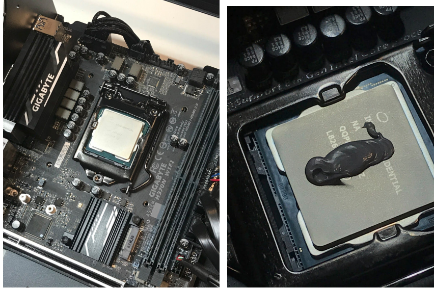
Fig. 37: A cleaned CPU core (left), reapplied Thermal paste on the core (right).
