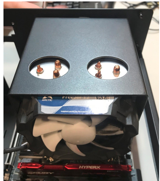
Fig. 18: Removing CPU Cooler Shroud thumbscrews (left). Internal view of the CPU Cooler Shroud (right).
