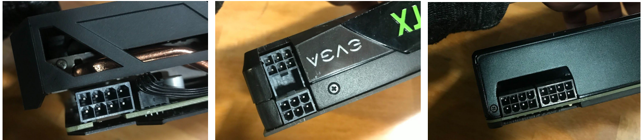
Fig. 30: Showing variations of pin connections on GPU cards - 8-pin (left), 12-pin (middle), 16-pin (right).
