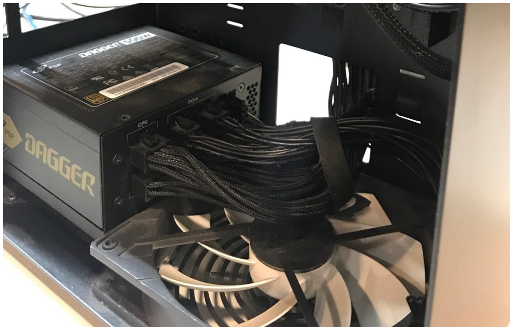
Fig. 29: Power supply cables tied together with supplied velcro strap, above chassis fan.
