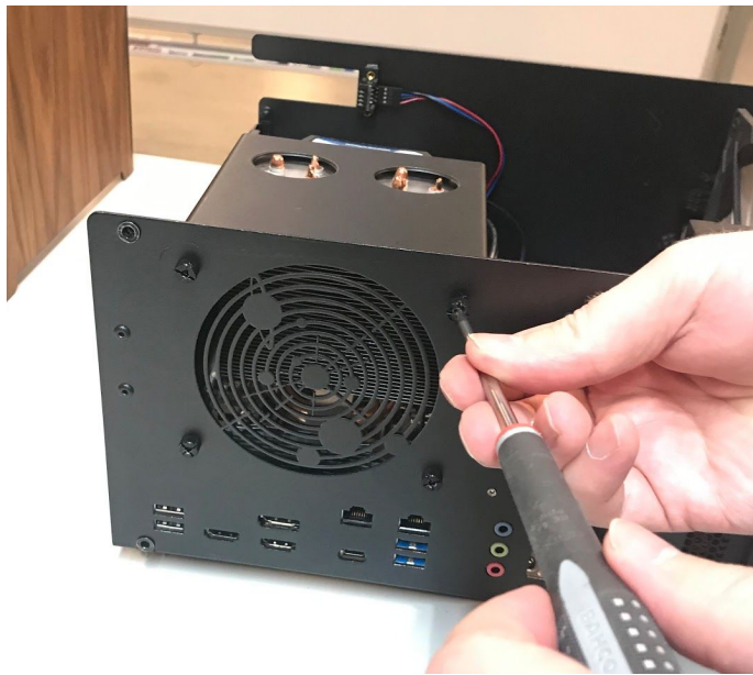
Fig. 18: Removing CPU Cooler Shroud thumbscrews (left). Internal view of the CPU Cooler Shroud (right).
