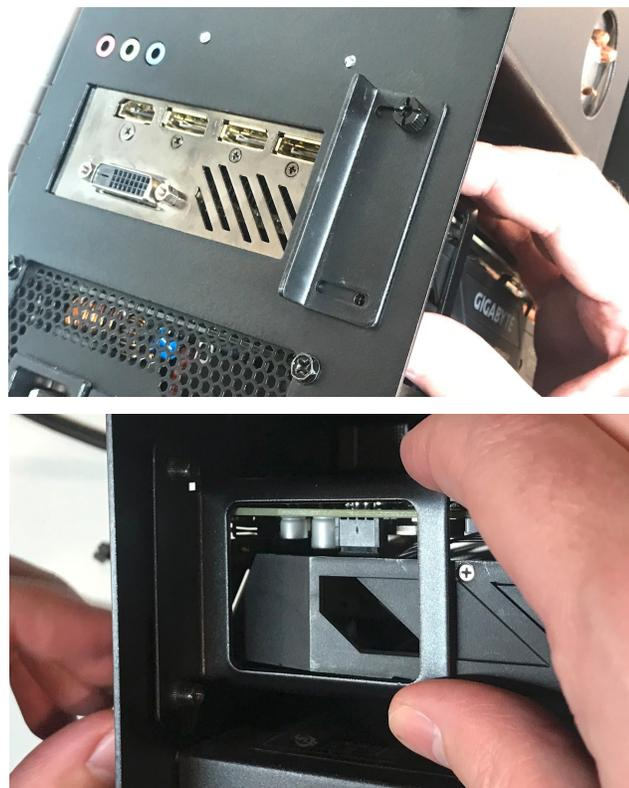
**Fig. 23:** Removing the thumbscrews and GPU Bracket.
