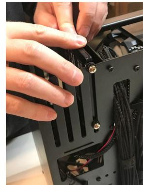
The internal M.2 storage drive is situated somewhat behind the GPU in the chassis. If you install an M.2 drive in this slot, you may need to [remove the GPU](#) beforehand to free up space. You can find video instructions on this process [here](#). If your Thelio has only one M.2 drive, or do not have a GPU installed. You can simply unscrew the M.2 drive from the chassis, without needing to remove a GPU.
