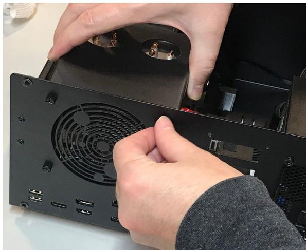
**Fig. 20:** Replacing the CPU Cooler Shroud and thumbscrews.
