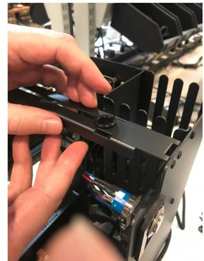
To add a 2.5-inch drive, you'll need 4 screws to secure the drive in place. We've provided screws for you on the chassis because we know just how easy they are to lose.
