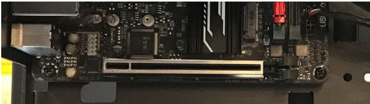
**Fig. 27:** Close up view of the PCIe slot.
