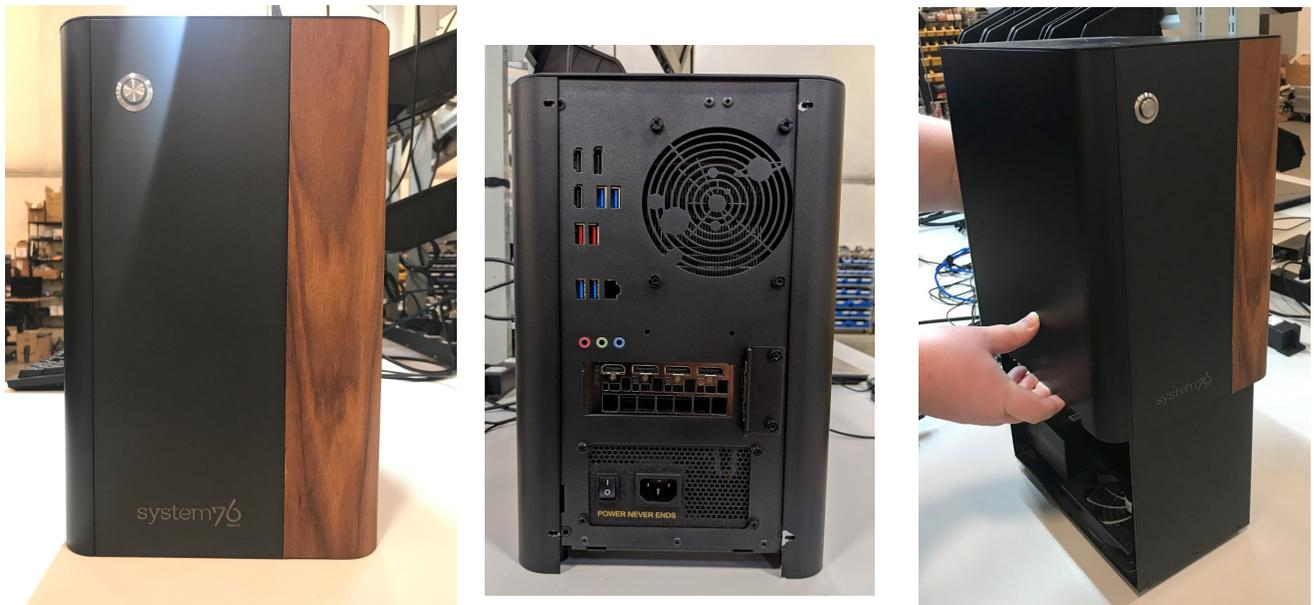
**Fig. 9:** Thelio Outer Case views, front (left), back (middle), Top Case partial removal (right).
