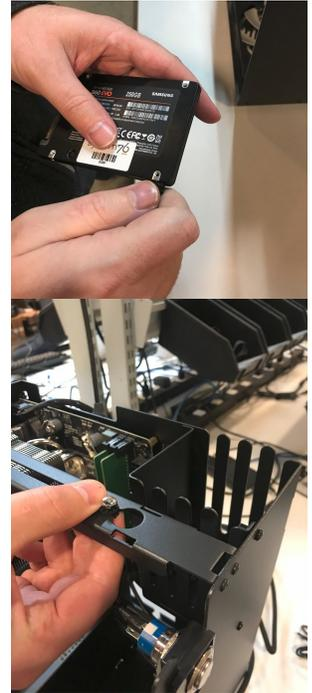
Fig. 31: (above and below-right) Sequence of shots showing the removal and/or replacement of 2.5" drives in the Thelio drive cage.
