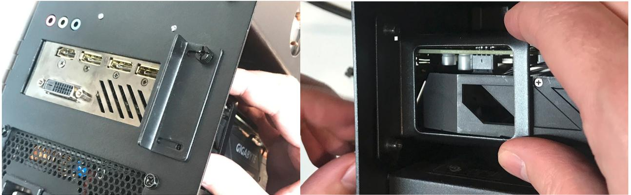
**Fig. 28:** Replacing the thumbscrews and GPU Bracket.
